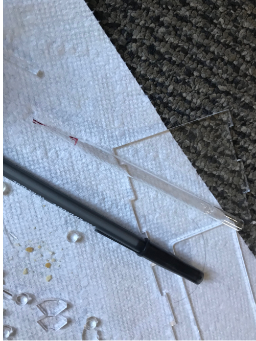
Figure 34: Acrylic Cutouts being removed from the sheet provided by Lux Lab. There were many small pieces, and devices like pens and tweezers were helpful.
