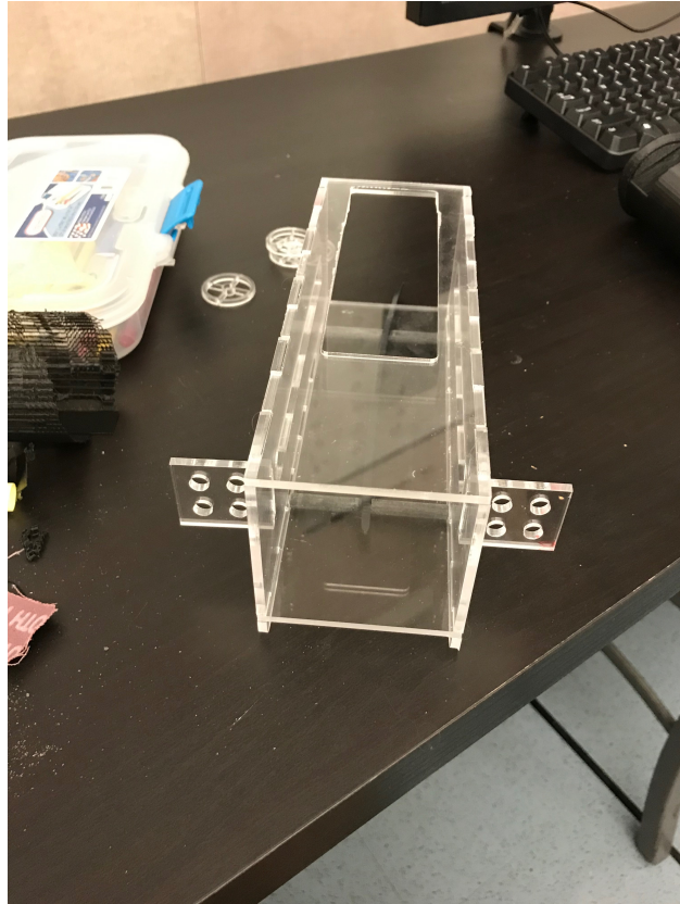
Figure 38: Partially assembled chassis. The rubber band holders were attached to the side walls using Scigrip 16, a glue specially made for acrylics that works by bonding acrylic to itself, creating an acrylic-like material that connects the acrylic, all while releasing flammable carcinogenic fumes.
