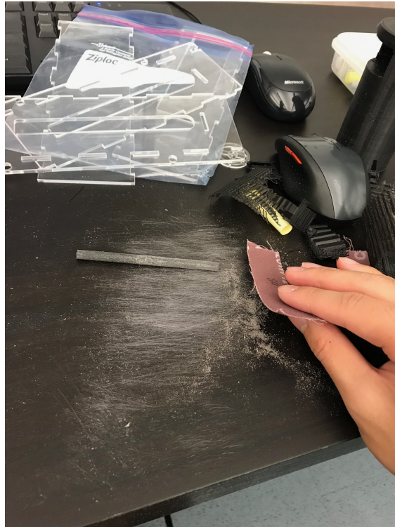
Figure 37: Sanding the axles to make them fit in the holes that were laser cut. The 1mm tolerance that I gave was not enough. My sanding technique was to start with 80 grit and work until the axle goes through the hole, then switch to 120 grit, and finally 180 grit.
