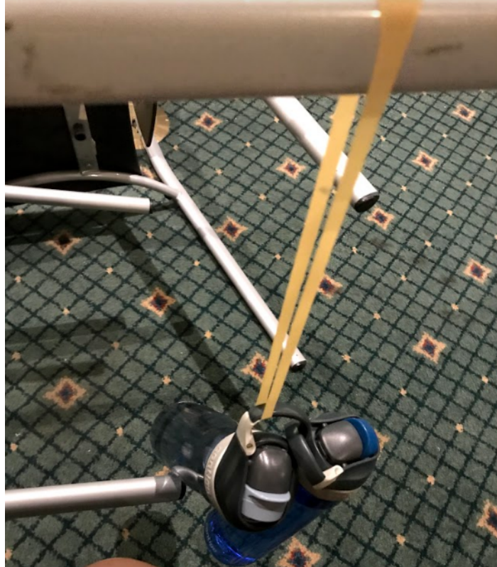
Figure 14: This picture shows the method used to measure k , the spring constant of the rubber band. I used calipers to make accurate measurements.
